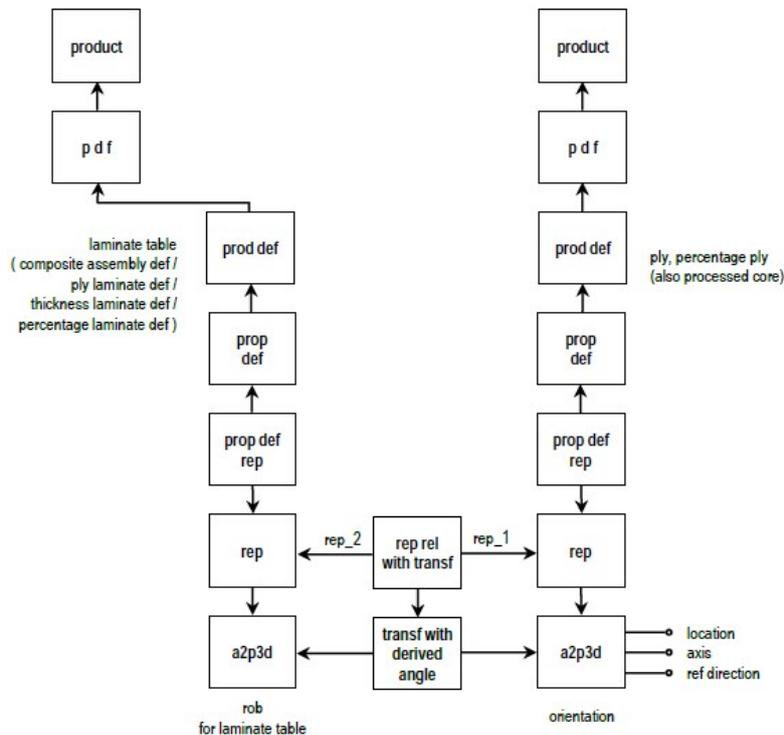
Figure 15: Ply Orientation by Simple Rosette
