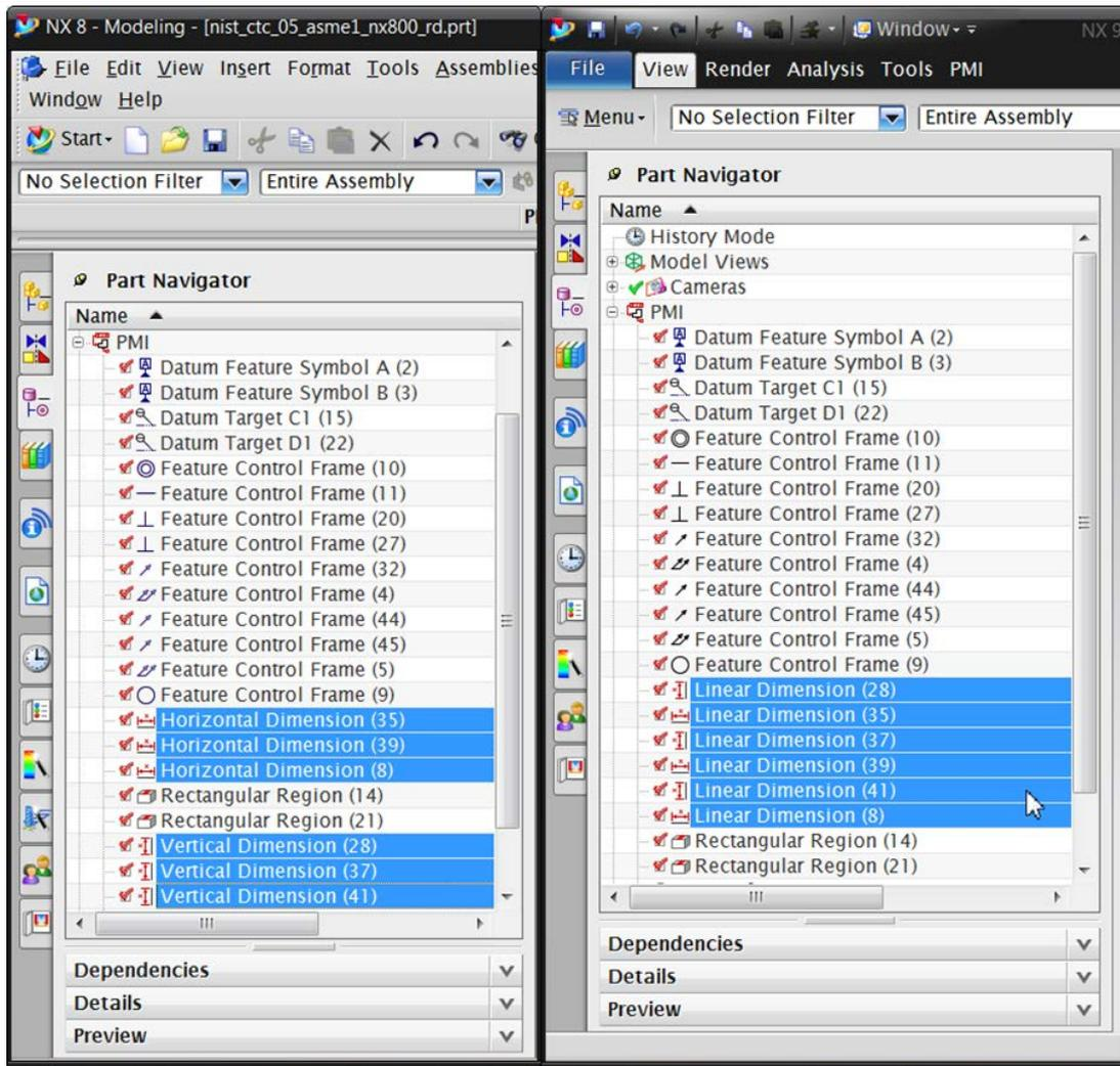
Figure 8: NX 8 vs. NX 9 Dimension Display Names
