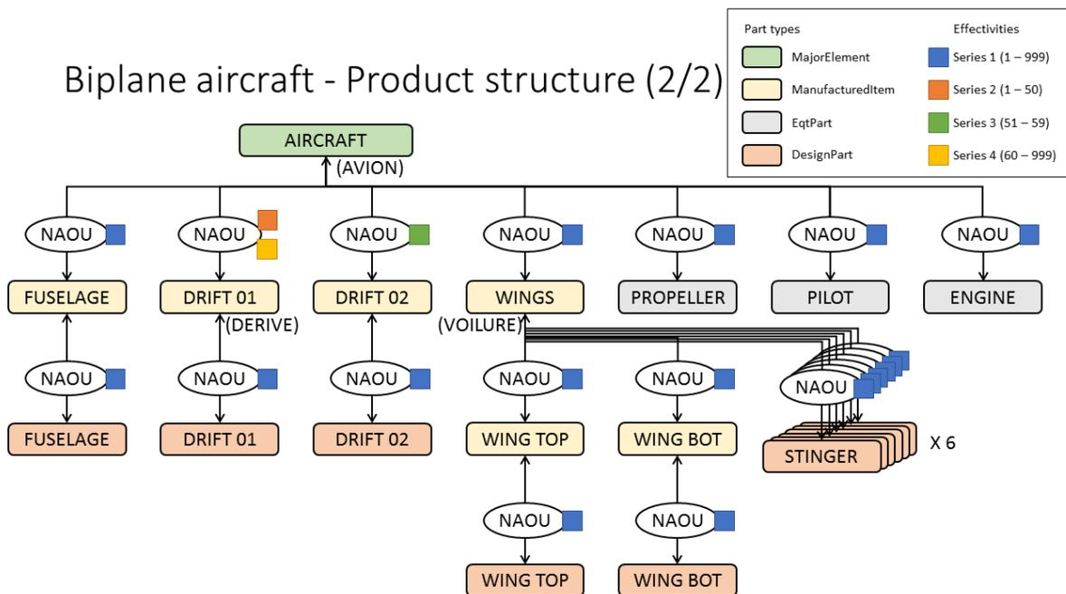
Figure 4: CONF2 Assembly Structure
