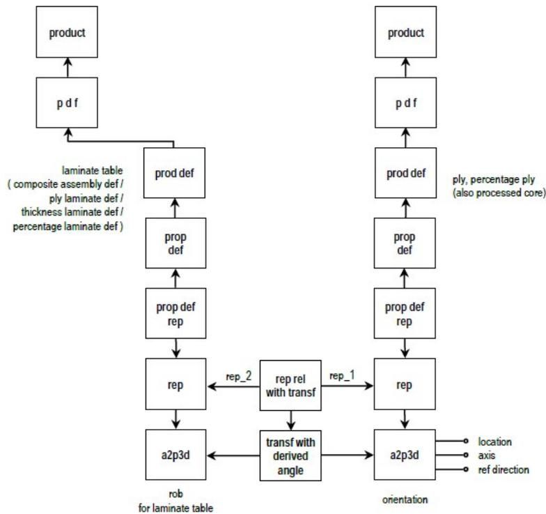
Figure 15: Ply Orientation by Simple Rosette
