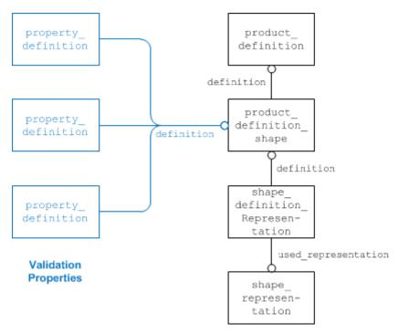
Figure 1: Validation Properties at the Part/Product level
