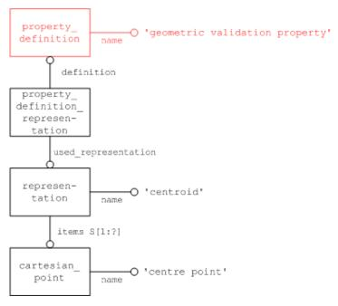
Figure 6: Geometric Validation Property "Centroid"
