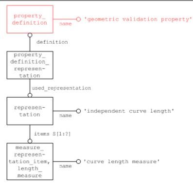
Figure 7: Geometric Validation Property "Independent Curve Length"
