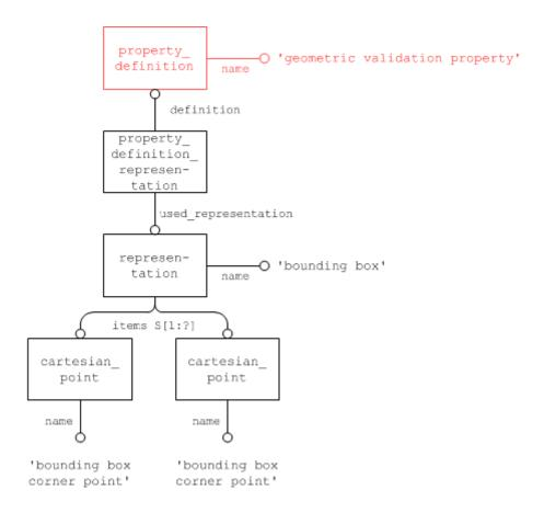
Figure 10: Geometric Validation Property "Bounding Box"
