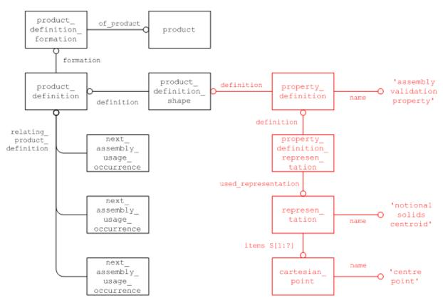
Figure 18: "Notional Solids Centroid Position" Validation Property
