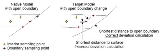
Figure 15: COPS – Sampling Points for an Open Boundary
