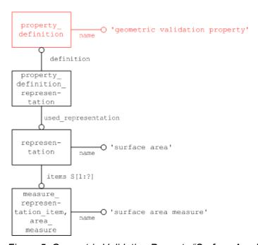
Figure 5: Geometric Validation Property "Surface Area"
