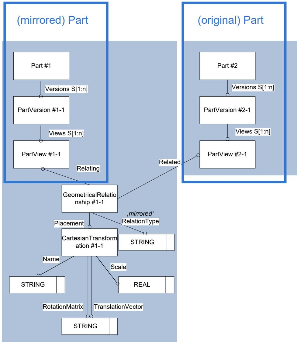
Figure 45: Template "Simplified Mirroring Positioning Representation"
