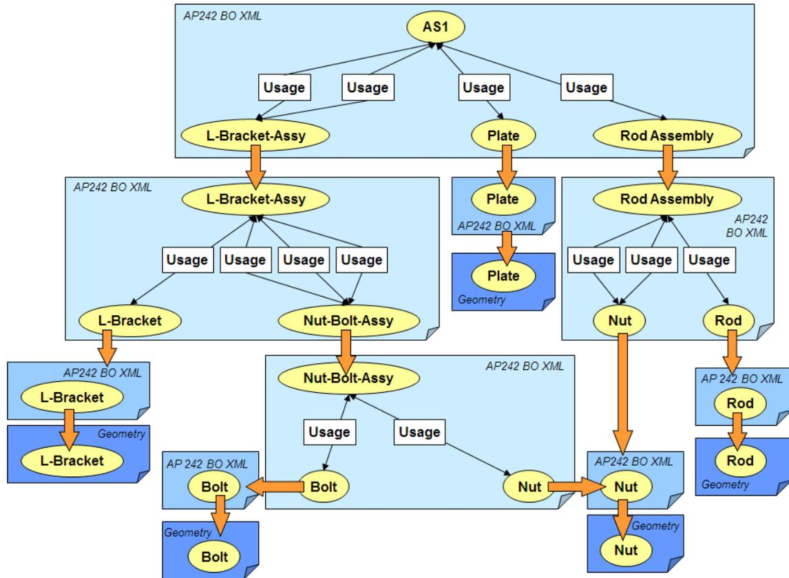
Figure 56: Example for Nested Structure with additional part-level XML files
