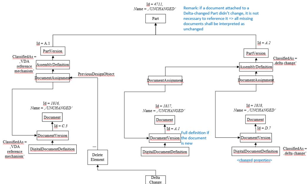
Figure 68: Example of the minimal instantiation of Delta Exchange of a new part version with one document deleted, one added and one modified
