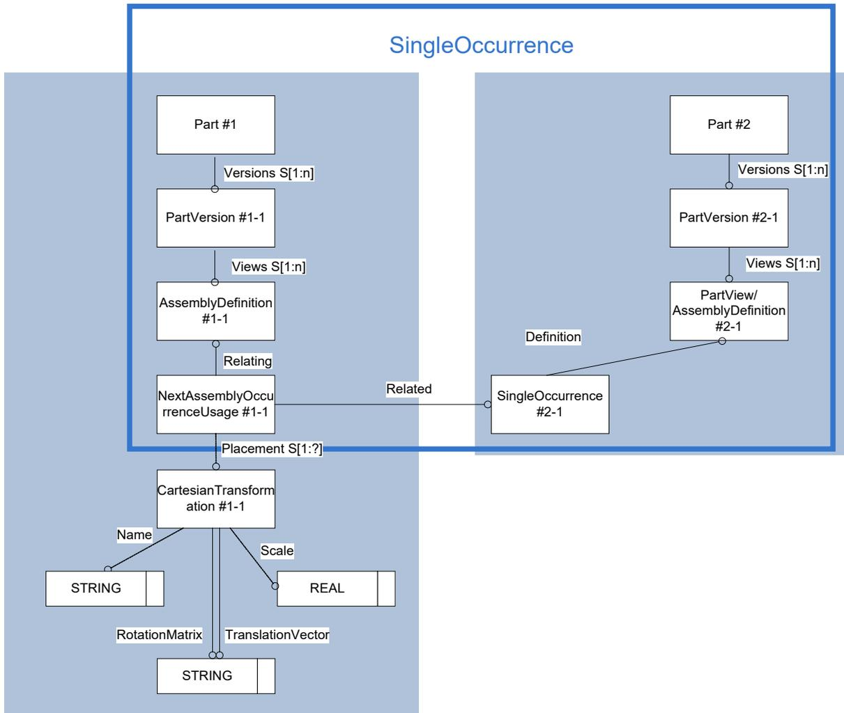
Figure 33: Template "Simplified Positioning Representation"
