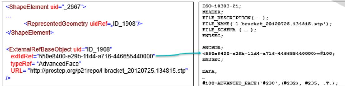
Figure 72: Example of an EER to an element within a Part 21 geometry file
