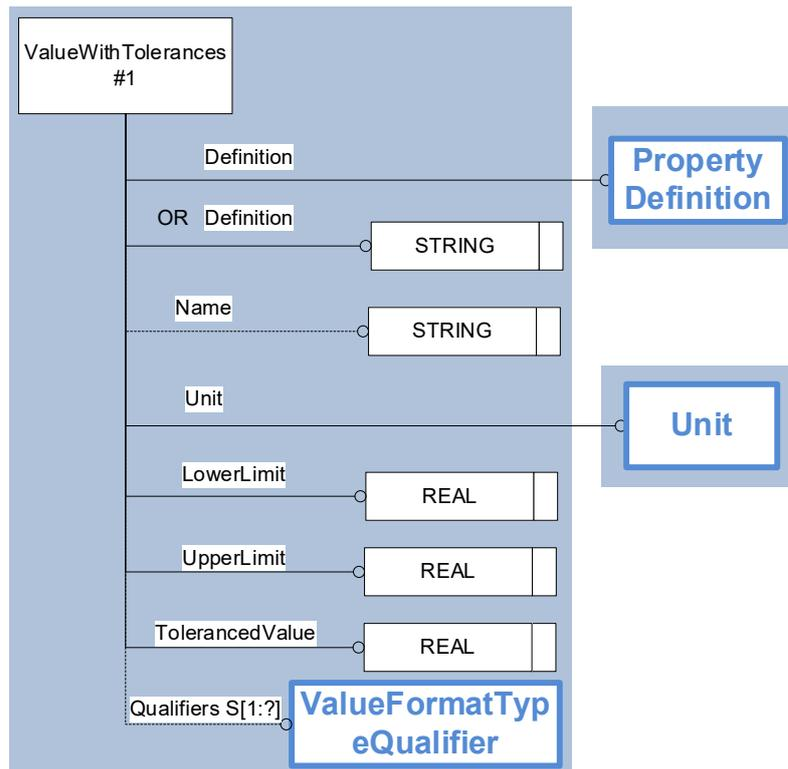
Figure 12: Template "ValueWithTolerances"
