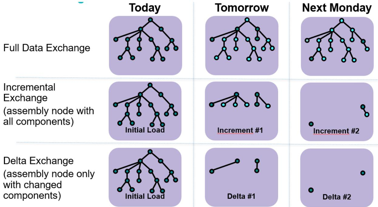
Figure 64: Differences between full data exchange, incremental exchange and delta exchange
