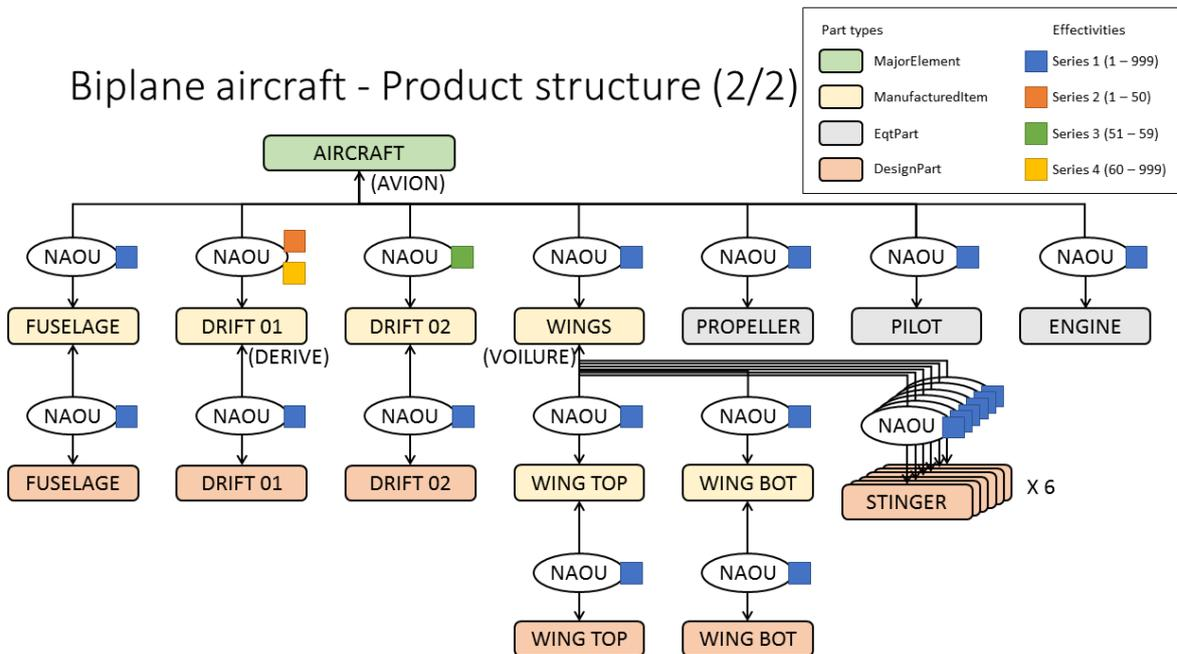
Figure 4: CONF2 Assembly Structure
