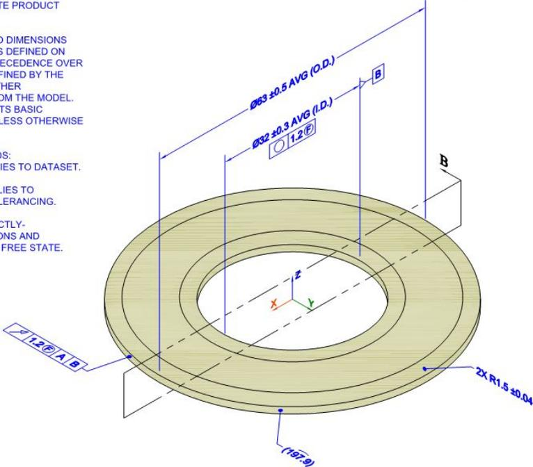
PMI Fully-Toleranced Test Case 11 - View A
